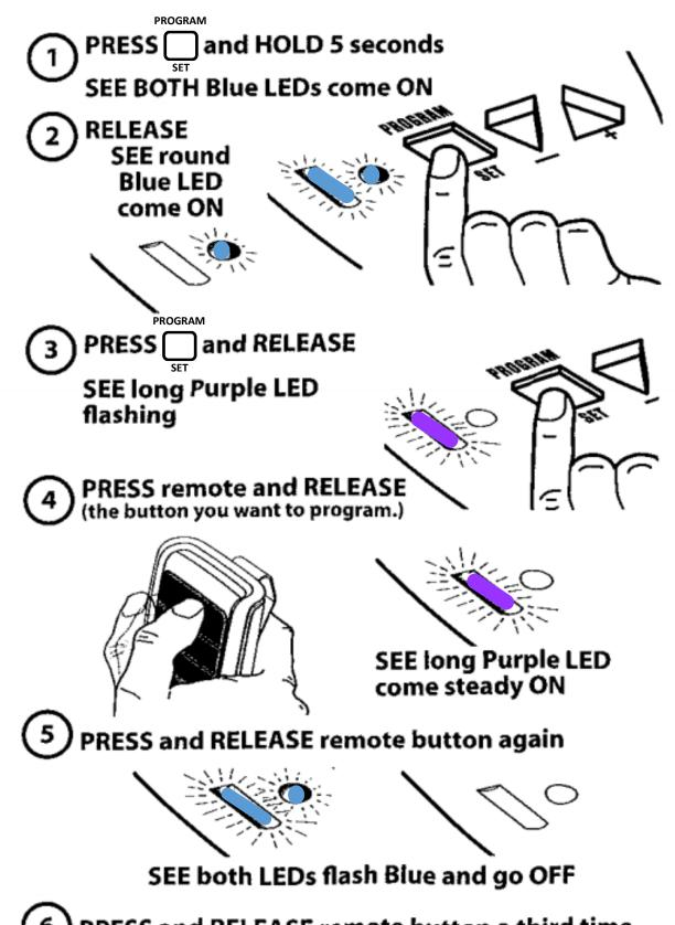
Programming is complete. This remote button can now be used to operate door opener.
